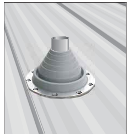
Fig. 13 Pipe Boots provide a watertight seal around roof vents and come in a variety of sizes. They seal with caulk under the base and around the pipe. To assure water tightness of the roof, avoid installing over panel ribs.
