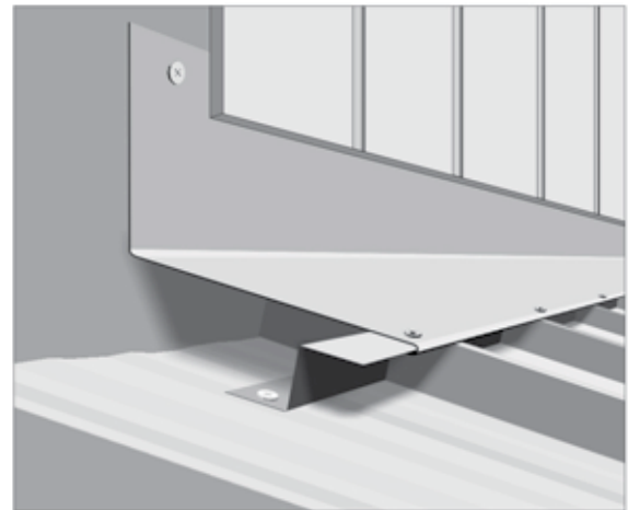
Fig. 18 Endwall flashing is applied where the upper slope of a roof meets a wall.
